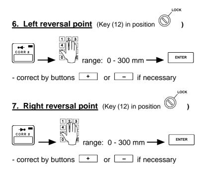
If the wire guide occurs inside of the winding window (between left and right reversal point), its direction can be programmed as follows
