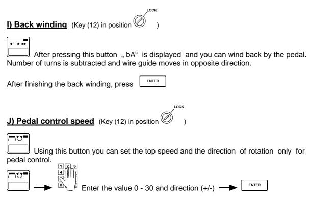
This speed and direction of rotation is then valid for all the processes controlled by the pedal.
